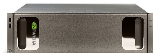
Nvidia DGX-1 8x Tesla V100, 3.2 kW 170 Tflop/s, 128 GB
